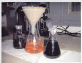
Left: original dark solution Center: lead clarified sample Right: celite filtrated sample in Autofilt
