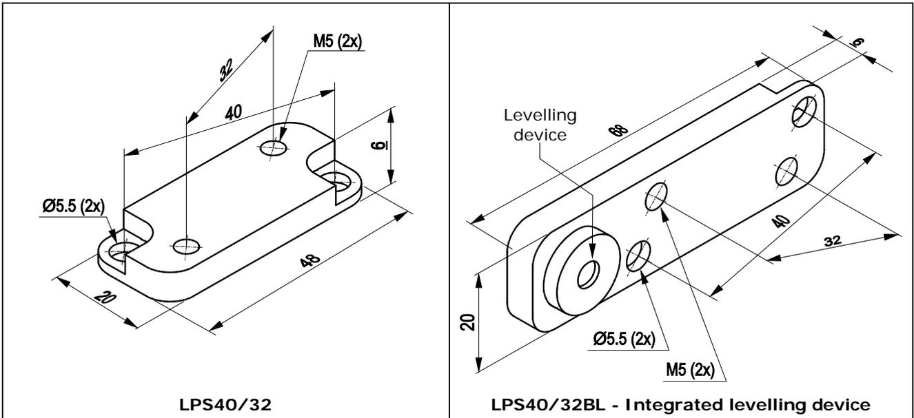
**Fig. 3.2: fixing adapters from 40 to 32 mm holes centre distance**
