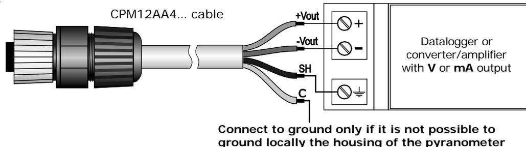
**Fig. 4.1: LPPYRA-Lite connections**
